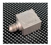
The GVT10S-T is a general purpose triaxial IEPE accelerometer for the measurement of broad band vibration in a wide range of vibration test applications, its small size and low mass make it an ideal all rounder. The tapped base means it can be stud mounted or used with an adhesive base (KMS-ADH1 or KMISO-ADH).
