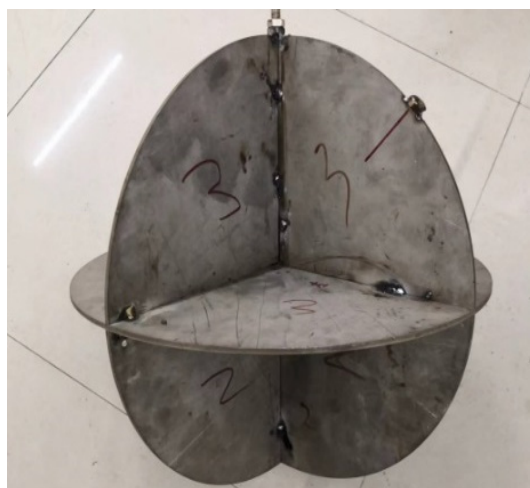
Figure 22. Eight-grid steel plate corner reflector.
