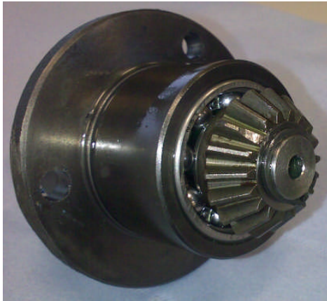
Figure 5. The gear with partly missing tooth.
