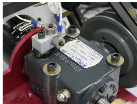
Figure 4. The gearbox with installed accelerometers.
