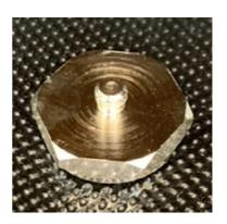
The KMMAG-21S is an isolated magnetic mounting base for use with accelerometers and other sensors requiring surface mounting. It features a nickel plated mild steel body and a PTFE isolating washer. This solution solves issues of earth loops causing interference in data signals from sensors.
