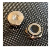
The KMMAG-14 is an isolated magnetic mounting base for use with accelerometers and other sensors requiring surface mounting. It features a nickel plated mild steel body and a PTFE isolating washer. This solution solves issues of earth loops causing interference in data signals from sensors.
