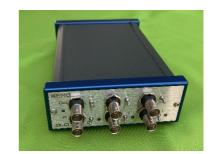
The 3X-CI is a 3 channel IEPE and charge signal conditioning unit, housed in a compact and rugged chassis. Featuring DC power input it can be used via the supplied mains DC adaptor or via a field based DC supply such as battery.
