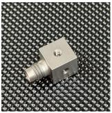
The SVT100S-T is a miniature triaxial IEPE accelerometer for use where mass loading is potentially an issue and should be minimised. At just 11.5mm cube and 5.8 grams it has an excellent frequency response. Tapped on two sides for ease of mounting.
