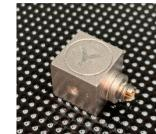
The MVT200S-T is a miniature triaxial IEPE accelerometer for use where mass loading is potentially an issue and should be minimised. At just 11.5mm cube and 10 grams it has an excellent frequency response with an increased sensitivity of 200mV/g which is ideal for measuring low level vibration or for use in Modal Testing applications.
