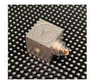
The MVT10S-T is a miniature triaxial IEPE accelerometer for use where mass loading is potentially an issue and should be minimised. At just 10.2mm cube and 4.2 grams it has an excellent frequency response.
