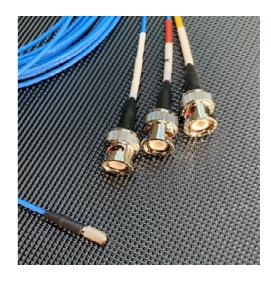
The 12F82-30 is a 3m compatible cable assembly developed for use with a range of triaxial accelerometers that use a miniature 8-36 threaded 4 pin connector. This can be seen typically on triaxial accelerometers such as the 356A30 and 356A22. Although it is also used on a range of other sensors.
