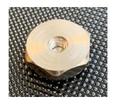
The KMMAG-21 is an isolated magnetic mounting base for use with accelerometers and other sensors requiring surface mounting. It features a nickel plated mild steel body and a PTFE isolating washer. This solution solves issues of earth loops causing interference in data signals from sensors.
