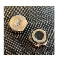
The KMMAG-14 is an isolated magnetic mounting base for use with accelerometers other sensors requiring and surface mounting. It features a nickel plated mild steel body and a PTFE isolating washer. This solution solves issues of earth loops causing interference in data signals from sensors.
