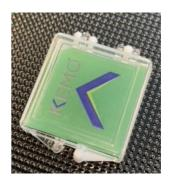
KMPWAX is petrowax supplied by Kemo Ltd for use with accelerometers and other sensor mounting. It is widely used for Modal testing where the user needs to move sensor locations regularly and the application requires limited frequency and amplitude measurements.
