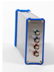
Two channel CardMaster 21.2 in compact mini rack.
